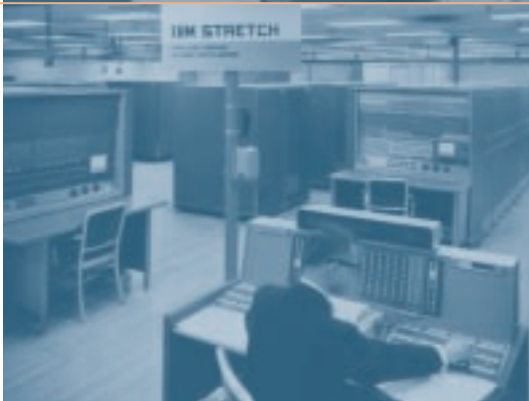
Stretch, an early IBM supercomputer, inaugurated the use of solid-state technology.
